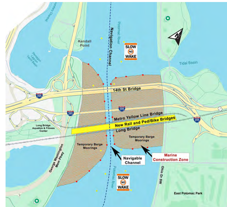
Aerial View of Marine Work Zone
